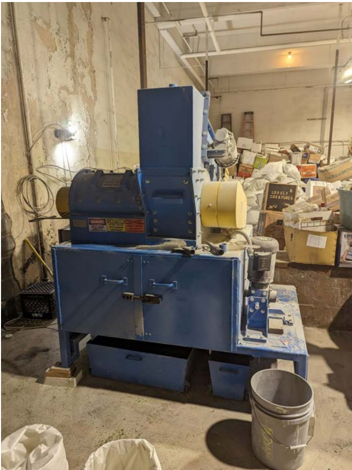
Figure 9: Andela GP Mini glass pulverizer installed at BU's facility.
