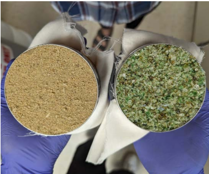
Figure 6: ASTM C-33 concrete sand (left) and glass-sand (right).
