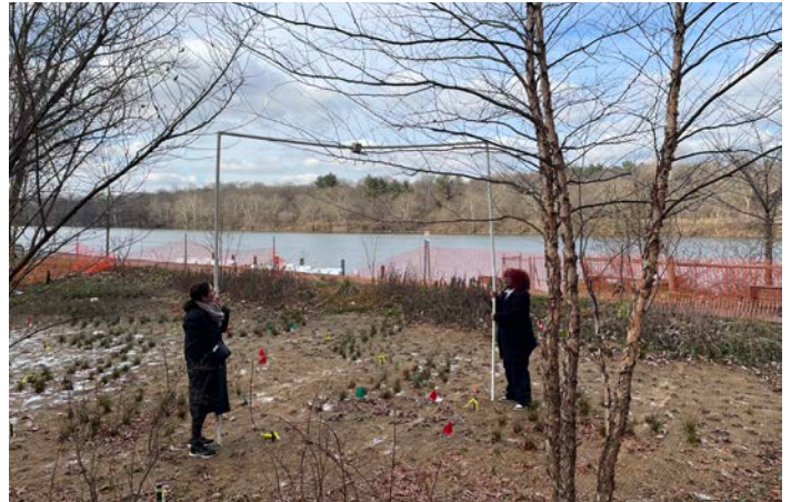
Figure 2: Overhead photograph being taken with photography rig.
